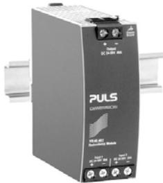
The YR40.482 is equipped with two input channels (20A each), which are individually decoupled by utilizing mosfet technology. The output current can go as high as 40A. Using mosfets instead of diodes reduces the heat generation and the voltage drop between input and output.
