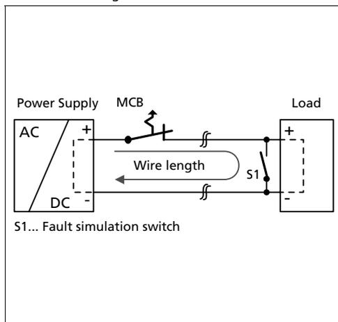
Maximal wire length<sup>\*)</sup> for a fast (magnetic) tripping:
