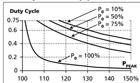
$$\text{DutyCycle} = \frac{T_{peak}}{T_{peak} + T_0}$$
