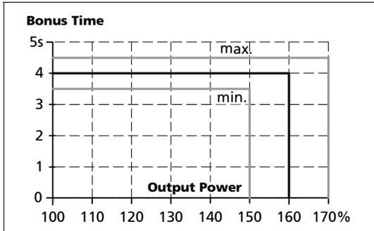
Fig. 6-4 **Dynamic overcurrent capability, typ.**
