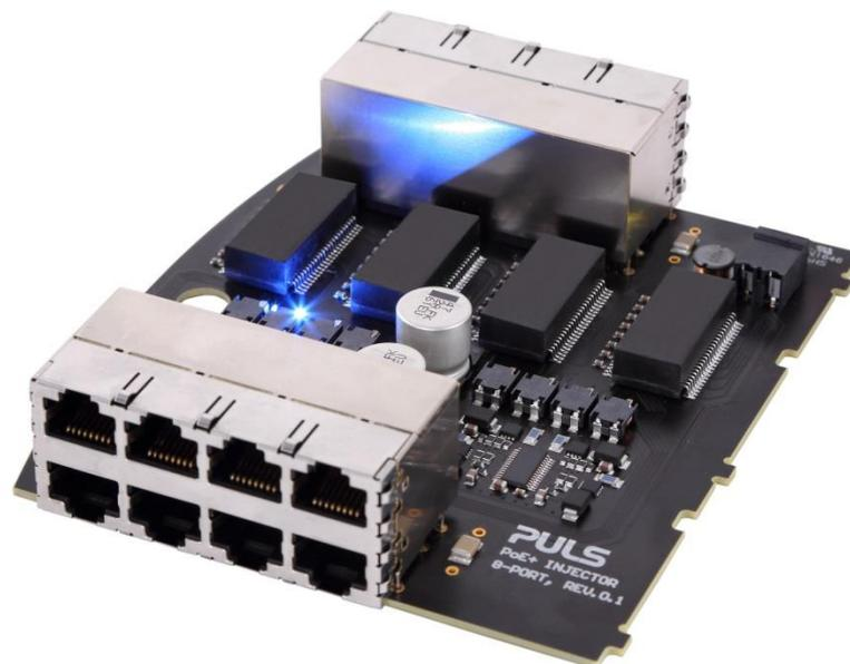
Figure 1: Power-over-Ethernet (PoE) injector - inner view
