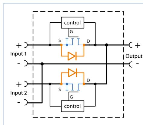
Image 2: Circuit design with Mosfet technology
