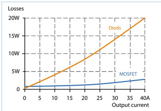
Image 1: A comparison of no-load losses of diode and Mosfet redundancy module (YR80.241)
