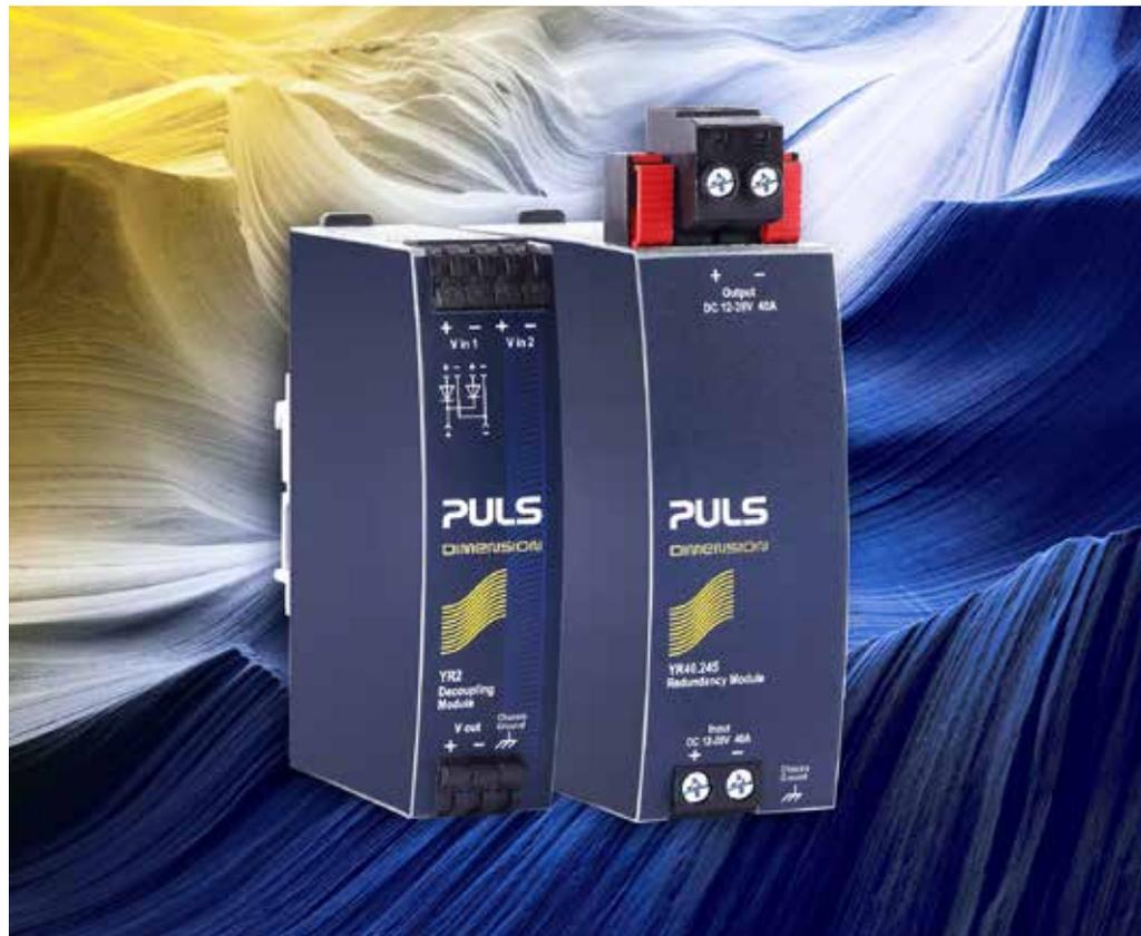
In a redundant system, two or more power supplies are switched in parallel and decoupled by one or more redundancy modules. The module prevents short-circuiting of the bus voltage if a short-circuit occurs in the output side of a power supply.
