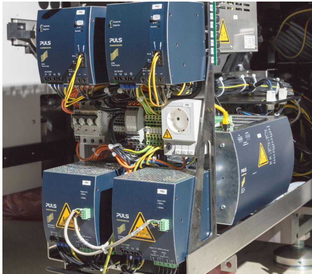
*Caption 1: For ASM, PULS has combined several standard power supplies, two modified power supplies and a purely client-specific assembly to a highly efficient complete system.*
