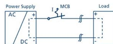
The resistance limits the current flow. Not more than the following current can flow in the event of a fault:  $I = U/R = 24V/1.195\Omega = 20A$
