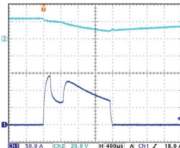
These curves were established with a QS10.241 (10A) power supply and 4A C Characteristic MCB. The upper curve is the output voltage with 20V/DIV. The lower curve is the fault current with 50A/DIV. A short peak current of approximately 145A flows
