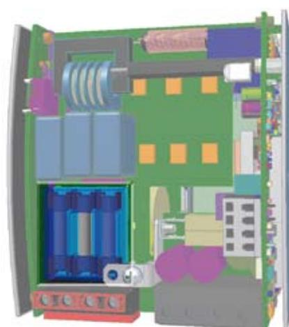
Figure 5: QT40 device with 3 in-built fuses save installation costs and space
