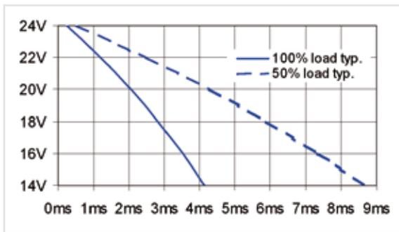
Figure 6: XT40: Buffer time depending on the output load
