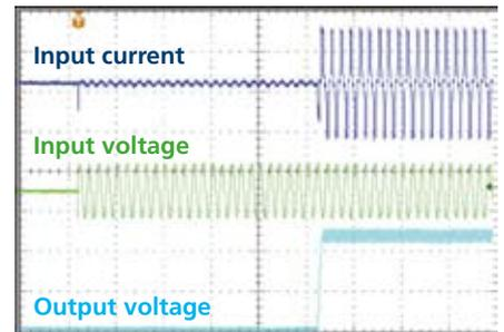
Figure 2: XT40; No inrush current surge when switching on
