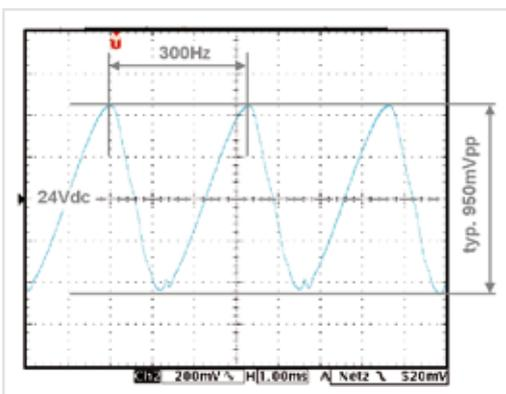
Figure 4: XT40: Ripple and noise voltage, 24V device
