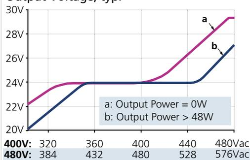
Figure 3: Output voltage regulation of the XT40 power supply
