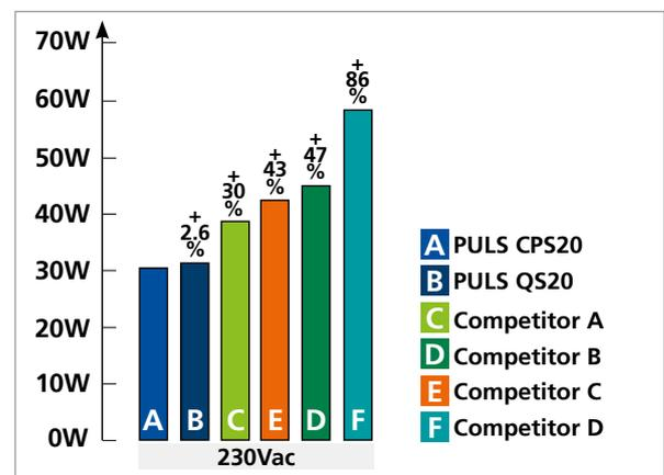
Figure 6: Comparison of the losses of different manufacturers of 24V, 20A single phase power supplies
