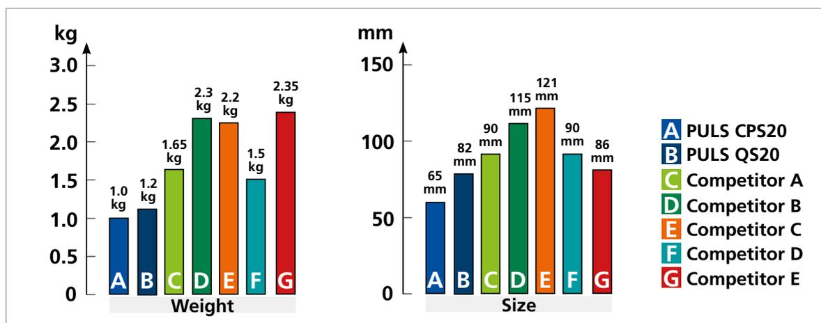
Figure 4: Comparison of size and weights of different manufacturers of 24V, 20A single phase power supplies
