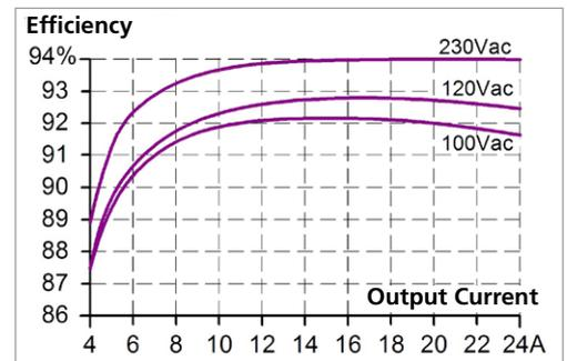
Figure 1: DIMENSION CPS20.241: High efficiency over a wide current range.
