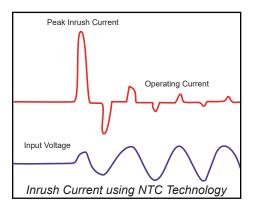
semiconductor resistors which show a decrease in resistance as temperature increases. A thermistor is a very simple way of controlling inrush for power supplies. When power is first applied, the thermistor is cold and has a high resistance, which limits the charging
