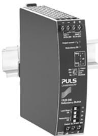
The YR20.246 is equipped with two input channels, which are individually decoupled by utilizing MOSFET technology. Using MOSFETs instead of diodes reduces the heat generation and the voltage drop between input and output. The YR20.246 does not require an additional auxiliary voltage and is self-powered even in case of a short circuit across the output.
