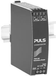
The YR20.242 is equipped with two input channels, which are individually decoupled by utilizing MOSFET technology. Using MOSFETs instead of diodes reduces the heat generation and the voltage drop between input and output. The YR20.242 does not require an additional auxiliary voltage and is self-powered even in case of a short circuit across the output.
