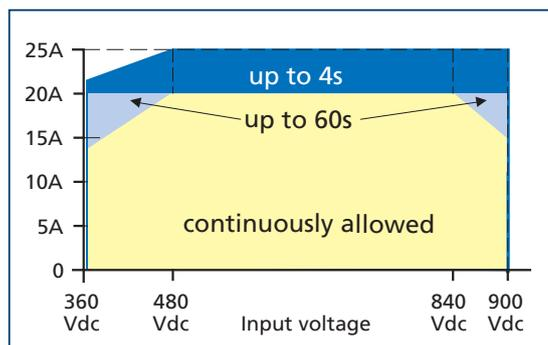
Figure 4: Allowed output current vs. input voltage
