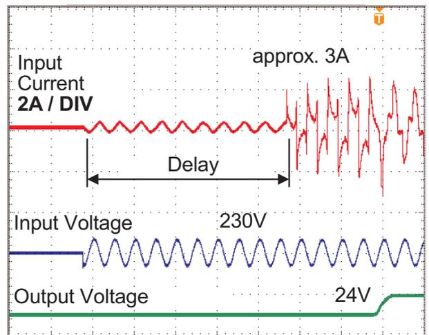
24V, 10A power supply from the PULS Dimension series with pulsed charging of the input capacitor
