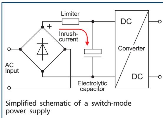
Simplified schematic of a switch-mode power supply
