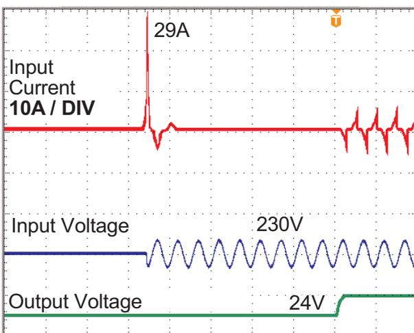
"Cold start" of a 24V, 10A power supply with NTC resistor inrush current limiting
