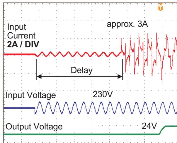
24V, 10A power supply from the PULS Dimension series with pulsed charging of the input capacitor
