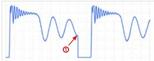
Valley switching: Switching at minimum voltage reduces losses
