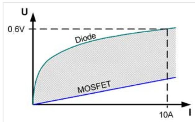
Voltage across the rectifier: Synchronous rectification with MOSFETs reduces the losses at full load about two-thirds.
