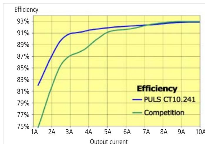
Increased efficiency in the partial load range via frequency-optimized control processes
