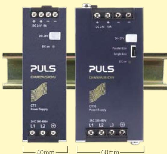
The CT5 Series is available with a 12V, 8A or a 24V, 5A output. The CT10 Series is available with a 24V, 10A or a 48V, 5A output.
