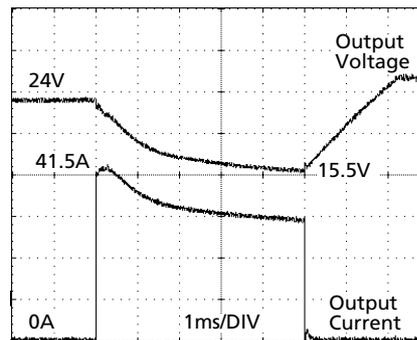
Fig. 23-3 **25A peak current for 12ms, typ. (3x the nominal current)**
