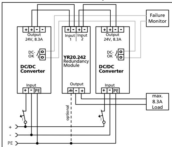
Fig. 23-5 Redundant power design utilizing the YR20.246 redundancy module with automated load sharing
