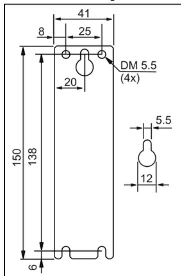
Fig. 22-6 Wall/panel mounting, side view
