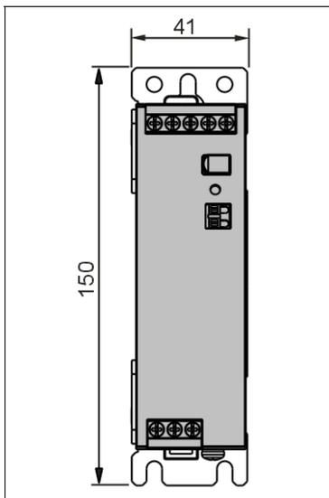
Fig. 22-5 Hole pattern for wall mounting
