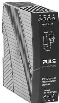
If 20A power supplies are utilized, it is recommended to connect the power supply output to both inputs of the redundancy module. Therefore, two redundancy modules are required to build a 20A redundant power system.
