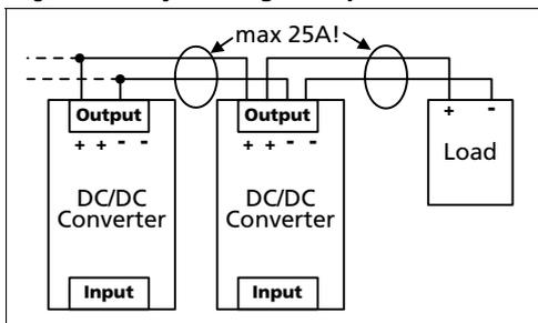
Fig. 13-3 Using distribution terminals
