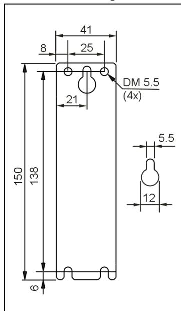
Fig. 23-9 Wall/panel mounting, side view
