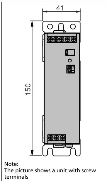
Fig. 23-8 Hole pattern for wall mounting
