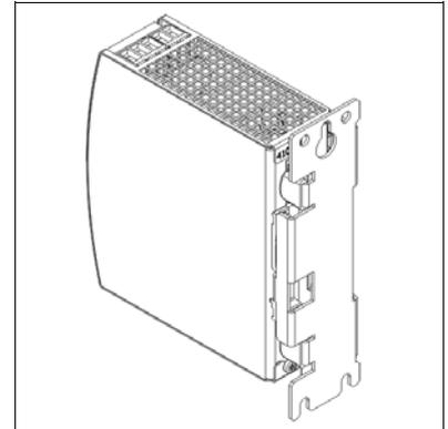
Fig. 23-7 Wall/panel mounting, front view
