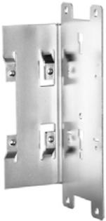
This bracket is used to mount the power supply sideways with or without utilizing a DIN-Rail. The two aluminum brackets and the black plastic slider of the unit have to be detached, so that the steel brackets can be mounted. For sideways DIN-rail mounting, the removed aluminum brackets and the black plastic slider need to be mounted on the steel bracket.
