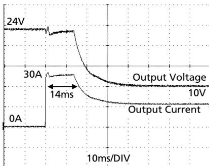
High Overload Current (typ. 25A for 12ms) enables easy fuse tripping
