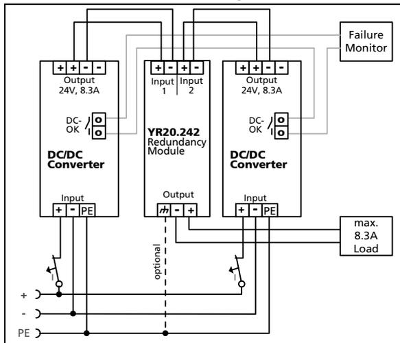
Fig. 24-7 Redundant power design utilizing the YR20.246 redundancy module with automated load sharing
