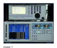
The efficiency of PULS switch-mode power supplies is measured with ultra-modern power analysers.
