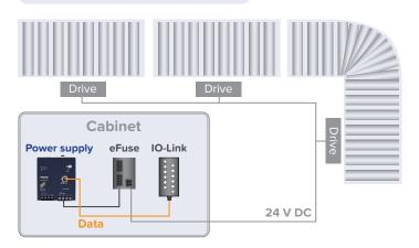
When relying on a centralized supply for the peripheral devices in the field, long cable harnesses with a large cross-section have to be taken into account. The power supply has to be oversized due to the associated loss of performance.
