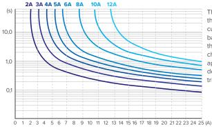
The graphic shows the characteristic curves that form the basis for shutting down the outputs. A different characteristic curve applies in each case, depending on the set tripping current.
